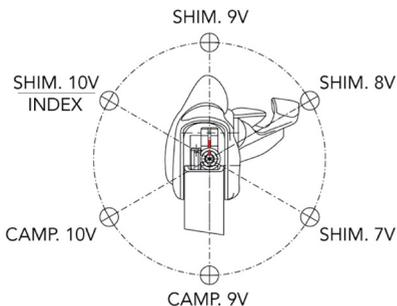
By simply working with a screwdriver from the front of the lever body, it is possible to change the speed system on the selector that runs straight through the lever. Both the brake and shift cables work in a straight line, reducing the risk of breakage due to repeated curving around a radius.
